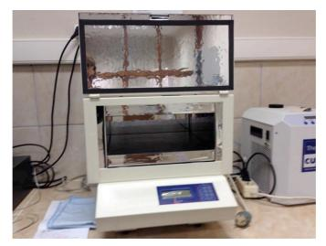
Figure 2. Lasercomp Fox-314 heat flow meter
