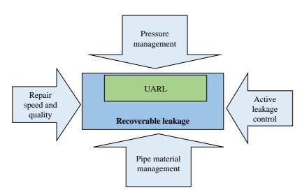
Figure 1: Basic reduction components of real losses [2]
