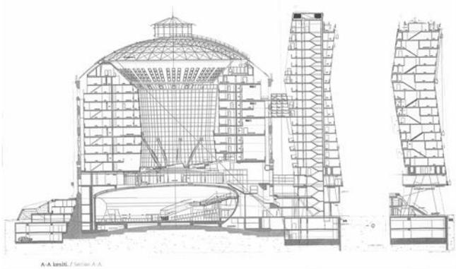
**Figure 9.** Cross-section view of Gazometre B structure with its shield-like new additional construction (Himmelb(I)au C., 2003).
