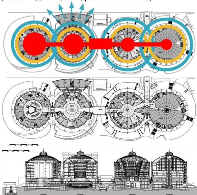
**Figure 3.** Ground floor plan and longitudinal section; plan and section drawings illustrating the spatial uses and the horizontal to vertical relationship of the Gasometer structures (www.gasometer.org, June 2005).
