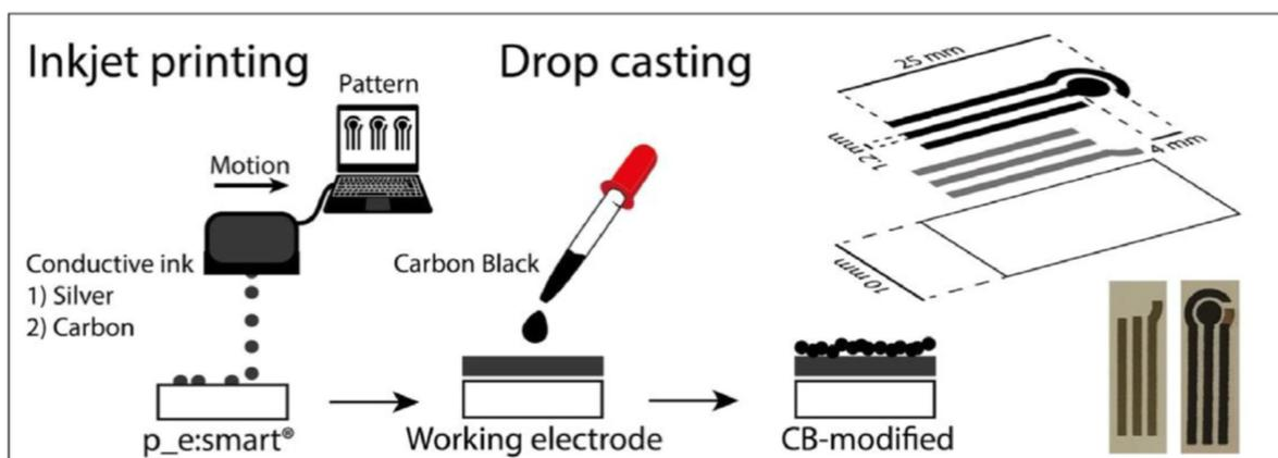
**Figure 4.** A schematic representation of paper-based inkjet printed electrodes production steps. Reproduced with permission from reference 59. Copyright (2018) Elsevier.
