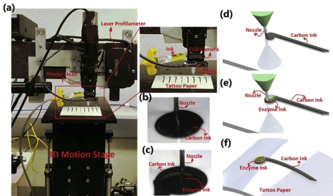
**Figure 3.** A schematic representation of direct-ink-writing of electrode and enzyme ink: (a) Custom-made direct-ink-write system, (b) direct-ink-write of carbon-mediated ink, (c) direct-ink-write of enzyme ink, (d) electrode printing, (e) enzyme printing, and (f) 3D printed electronics-based biosensor on a flexible substrate. Reproduced with permission from reference 57. Copyright (2018) Elsevier.
