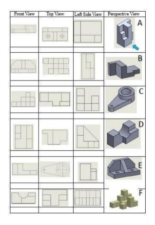
Figure 1: An Example For Which 3D Views And 3-Views Of The Parts Were Given For Question 1.
