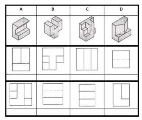
Figure 4: An Example For Which 3D Views And Views Of The Parts Were Given For Question 4.
