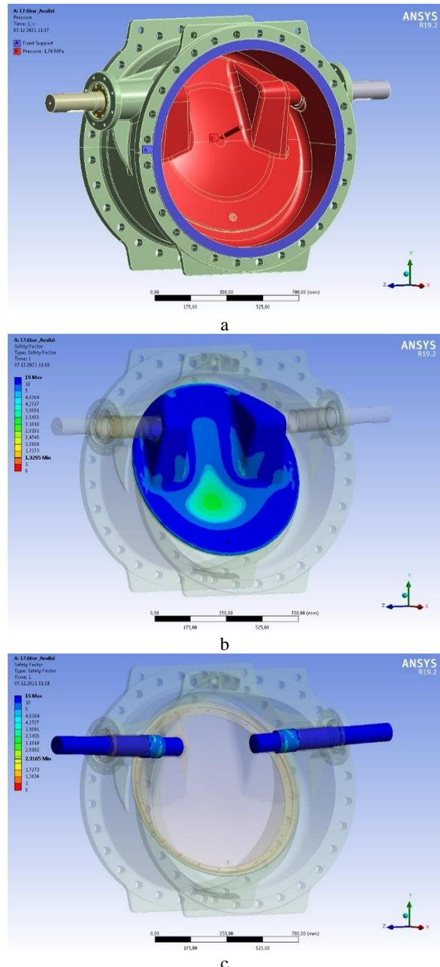
Figure 3. Assembled body, disc, and shaft's FEA analysis
