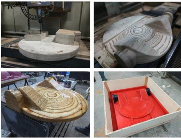
Figure 5. Pre-cast preparations of components' material
