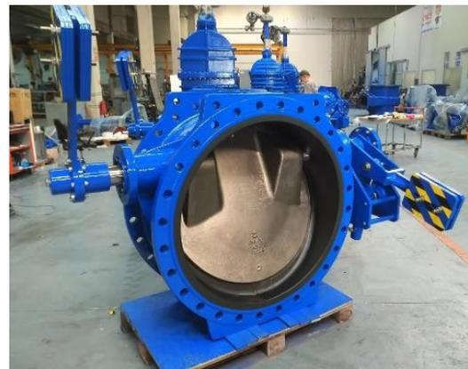
Figure 7. Prototype production of the developed design
