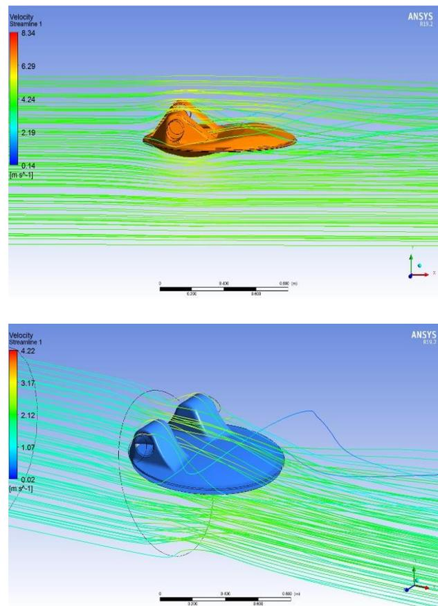
Figure 1. Velocity vector analyses of the design for front (upper) and isometric (below) views
