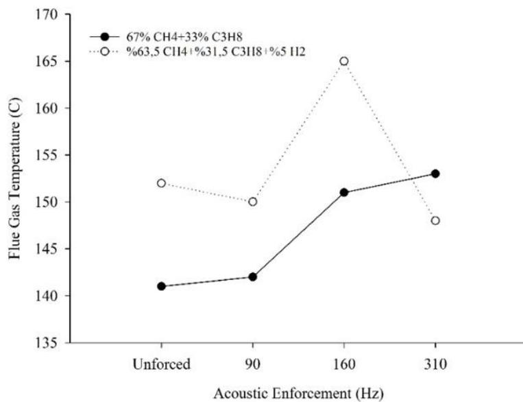
**Figure 5.** 2B flue gas temperature for different acoustic enforcement
