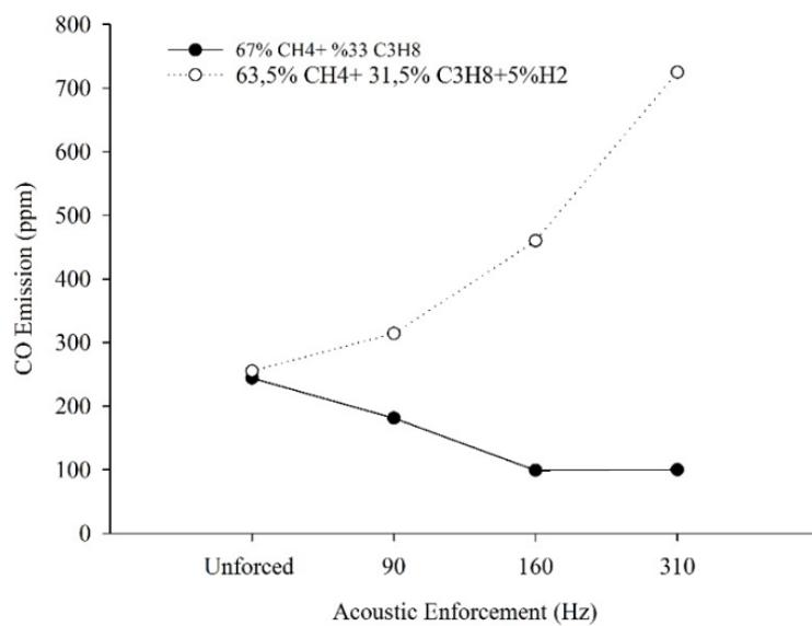
**Figure 9.** *CO* emission for different acoustic enforcement
