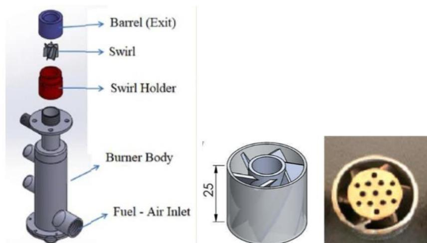
**Figure 3.** Burner and swirl generator detailed design
