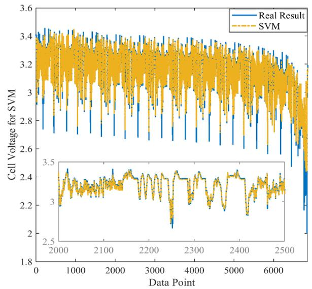
Figure 12. The fit of the  $V_T$  prediction value presented by FG-SVM.
