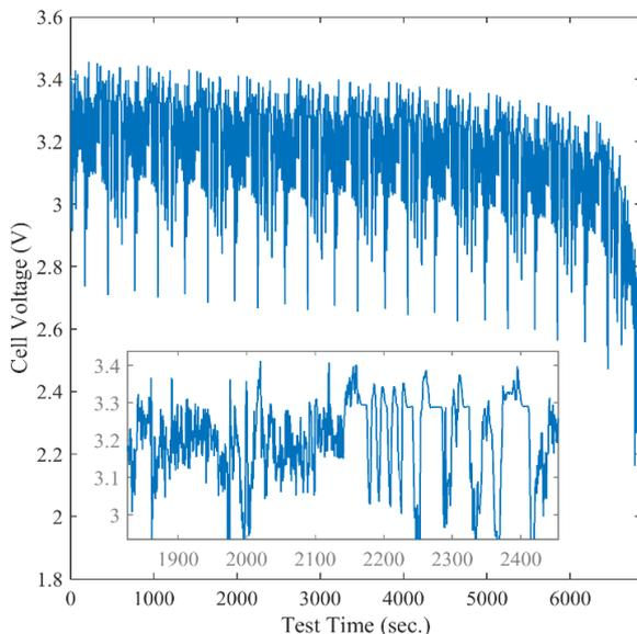
Figure 7. Changing of  $V_T$  according to current profile.
