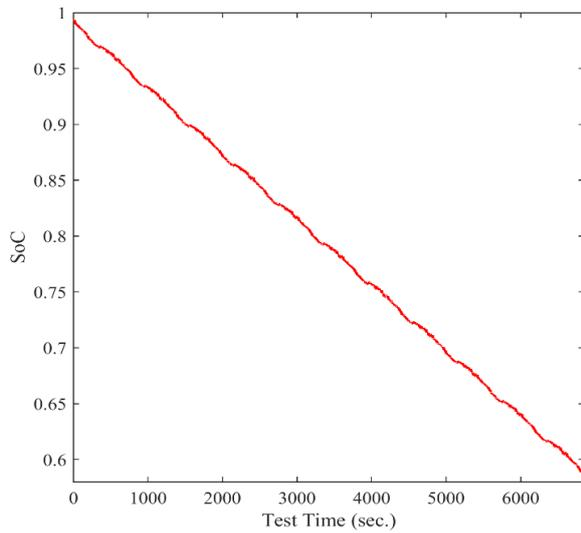
Figure 6. Variation of SoC according to current profile.
