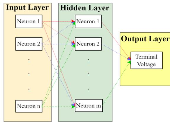
Figure 4. Layer structure and neuron connections of ANN.
