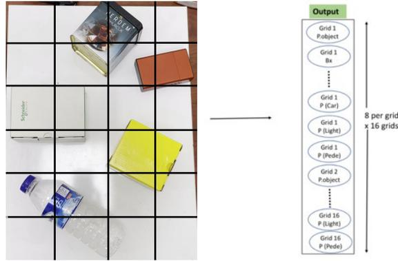
Figure 1: Structure of the YOLO algorithm
