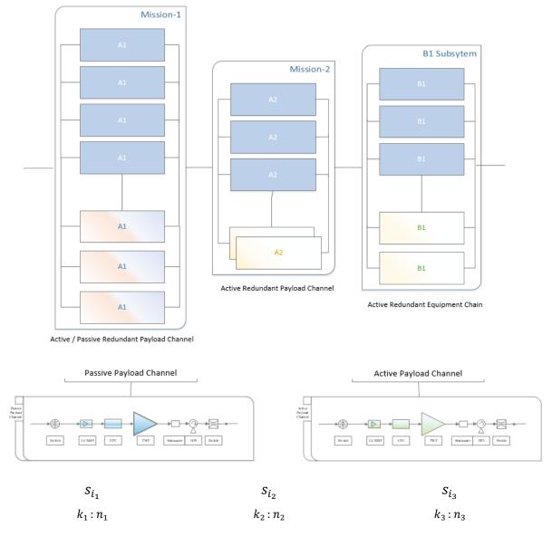
Figure 2. k-out-of-n Satellite Subsystems Reliability Block Diagram
