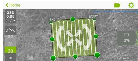
**Figure 7.** Flight plan for a height of 30 m
