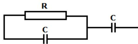
**Figure 11:** Tincal reinforced resin composites equivalent circuit diagram.
