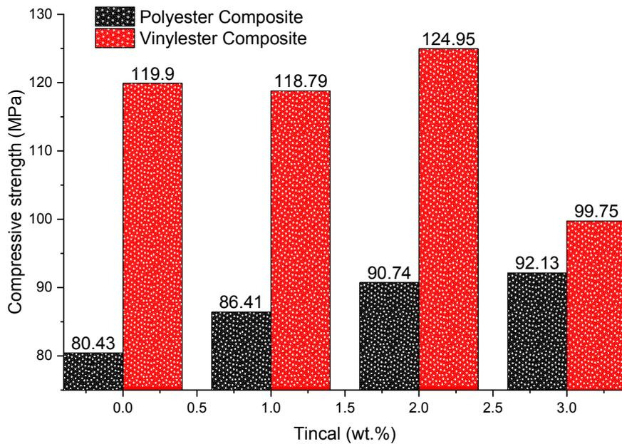
**Figure 6:** Compressive strength values of tincal reinforced resin composites.
