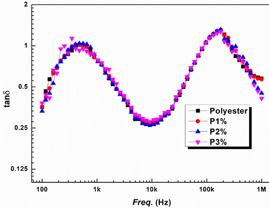
**Figure 9:** Dielectric properties of tincal-reinforced polyester composites.
