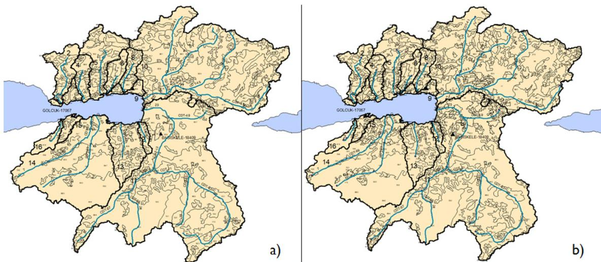
Fig. 5. Model of the basin, sub-catchments and drainage lines in the SWMM for a) 1990, b) 2012
