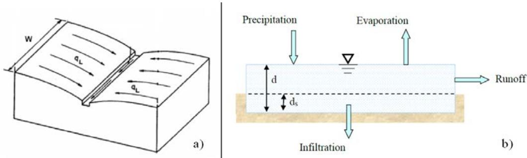
Fig. 4. a) Idealized representation of a sub-catchment b) Nonlinear reservoir model of a sub-catchment (Rossman and Huber, 2015)
