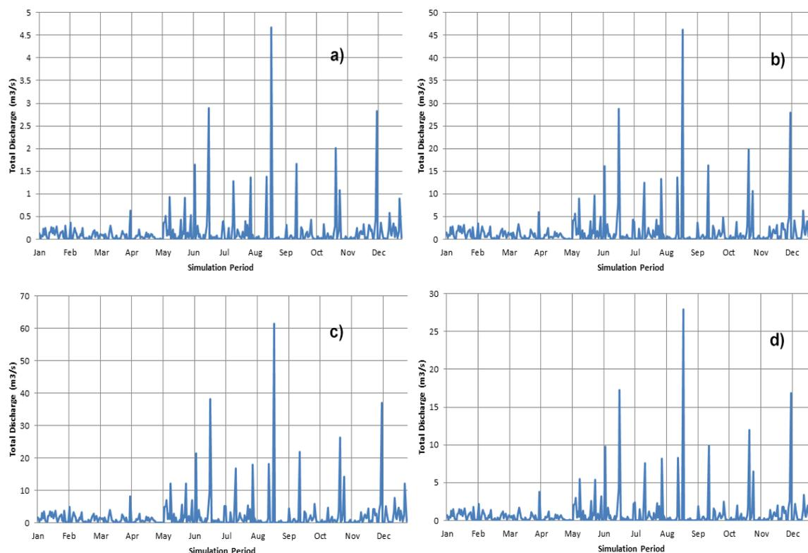
Fig. 6. Flow rates at outfall points of sub-basins 2 (a), 10 (b), 11 (c) and 14 (d) in the SWMM model of 1990
