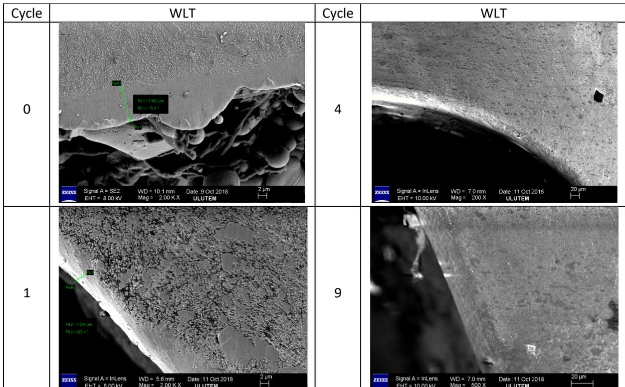
Figure 5. Removing of white layer during AFM
