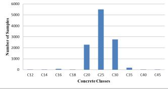
Fig 3. The distribution of the compressive strength of concrete produced in the provinces located in the first seismic zone of Turkey between 2006 and 2012
