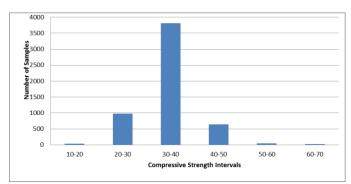
Fig 5. The number of samples belonging to some intervals of compressive strength (MPa) for C25 between 2006 and 2012
