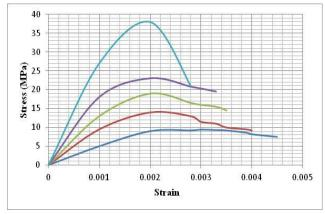
Fig 1. Stress-strain curves of concrete subjected to uniaxial compression [4]
