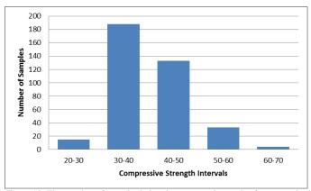
Figure 10. The number of samples belonging to some intervals of compressive strength (MPa) for C30 in 2013
