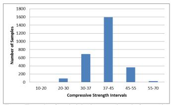
Figure 6. The number of samples belonging to some intervals of compressive strength (MPa) for C30 between 2006 and 2012
