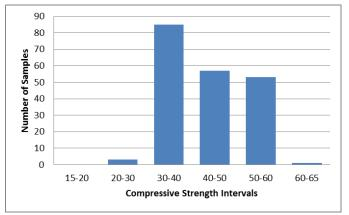
Fig 8. The number of samples belonging to some intervals of compressive strength (MPa) for C20 in 2013
