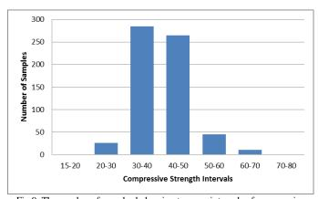
Fig 9. The number of samples belonging to some intervals of compressive strength (MPa) for C25 in 2013
