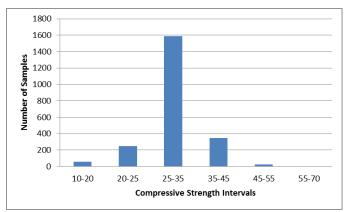
Fig 4. The number of samples belonging to some intervals of compressive strength (MPa) for C20 between 2006 and 2012
