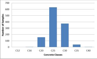
Fig 7. The distribution of the compressive strength of concrete produced in the provinces located in the first seismic zone of Turkey in 2013
