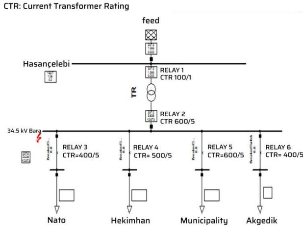
Figure 5. Example Transformer Substation Single Line update [25].
