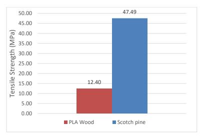
Figure 5. Average tensile strength values of test specimens
