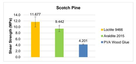
Figure 7. Shear strength of Scotch pine joints according to adhesive type
