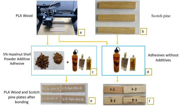
Figure 1. Flowchart of the adhesive bonding process
