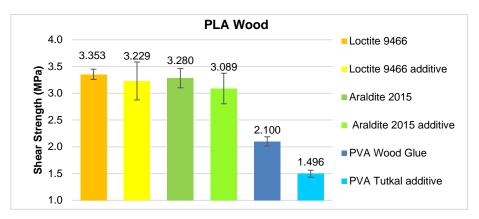
Figure 6. Variation of shear strength of PLA Wood joints according to adhesive type
