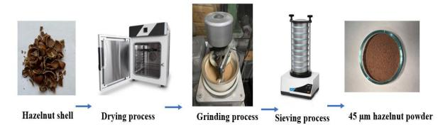
Figure 4. Hazelnut powder grinding process sequence
