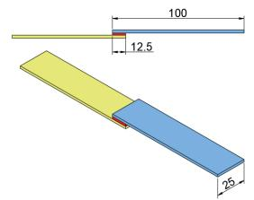
Figure 3. Single lap joint (mm)
