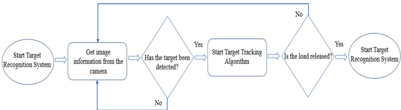
**Figure 9.** Target detection and recognition system algorithm flowchart
