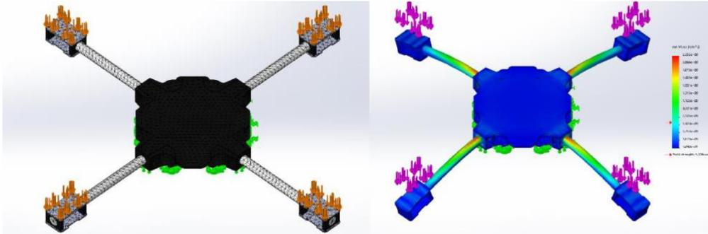
**Figure 4.** UAV Stress Analysis
