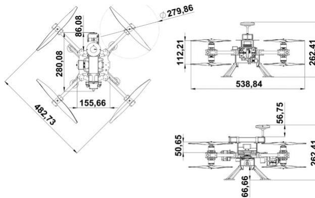
**Figure 1.** Dimensional parameters of the UAV
