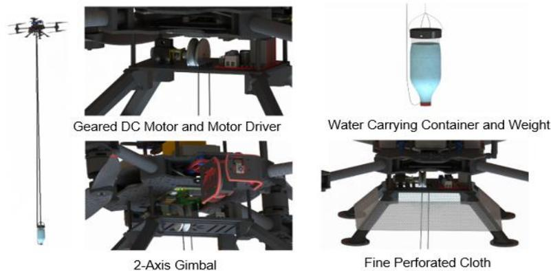
**Figure 6.** Task mechanism components
