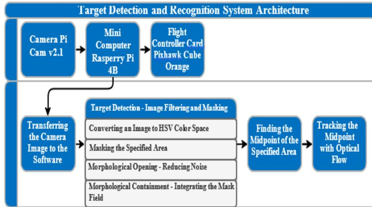
**Figure 8.** Target Detection and Recognition System Architecture
