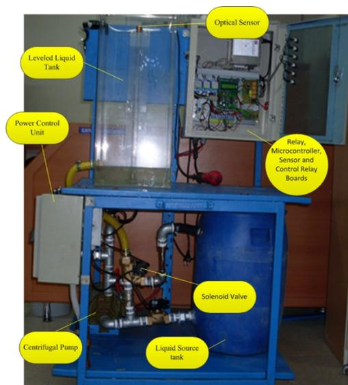
Figure 6. Mechatronic liquid level measurement system
