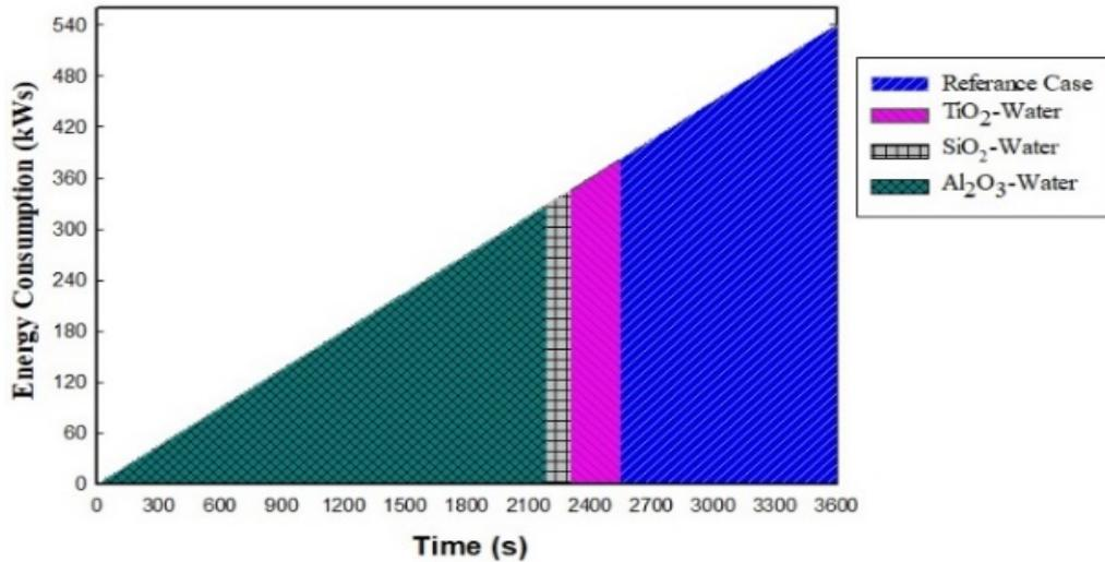
Figure 8. Comparison of electricity consumption with load conditions at 30 °C ambient temperature
