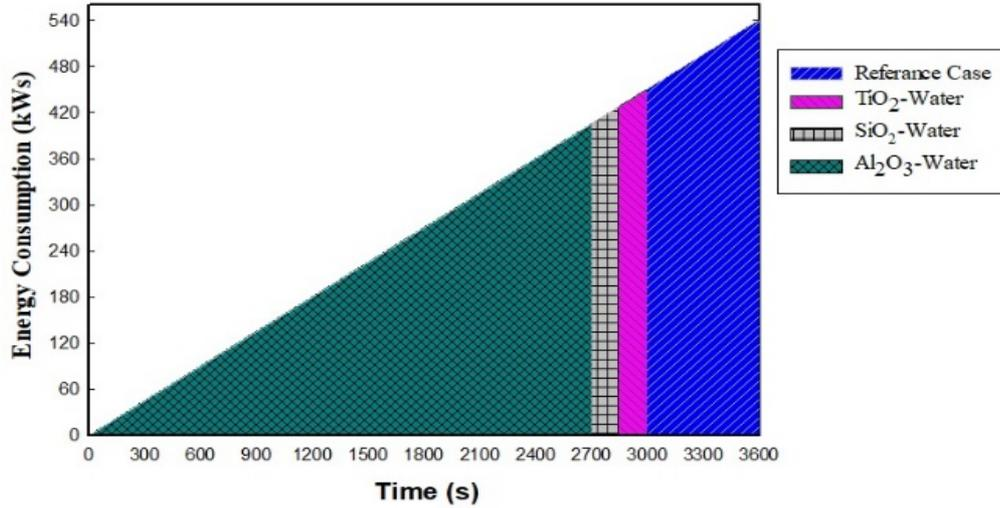
Figure 7. Comparison of electricity consumption without load conditions at 30 °C ambient temperature
