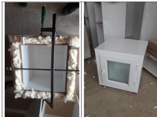
Figure 3. The production of the cooled cabinet
