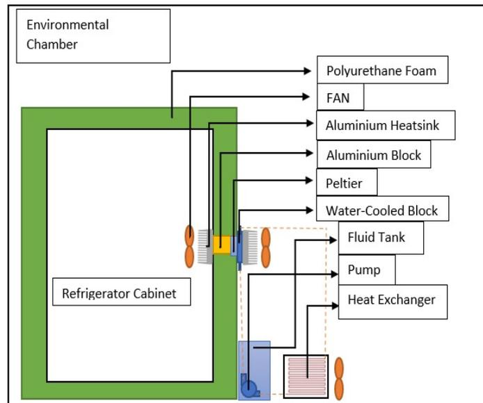
Figure 4. The schematic diagram of the TEC system
