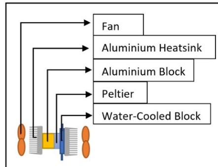
Figure 2. Schematic description of TEC systems
