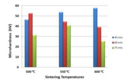
Figure 5. Microhardness values at different sintering temperatures and for different durations
