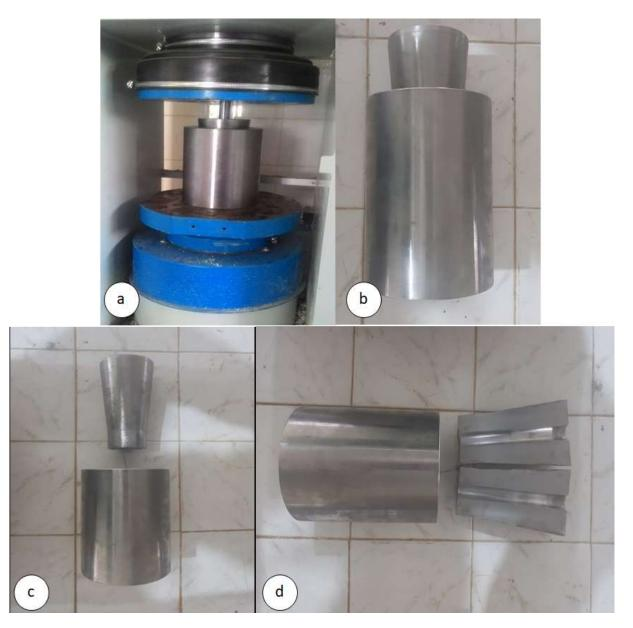
Figure 1. a) Pressing, b-d) Removal of samples following the pressing process
