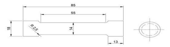
Figure 2. Tensile strength size (mm)
