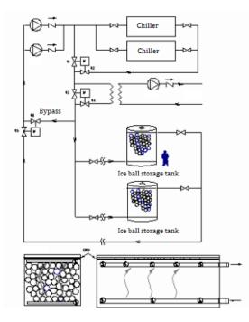
Figure 5. Spheral encapsulated thermal energy storage system (Iceball, [15])
