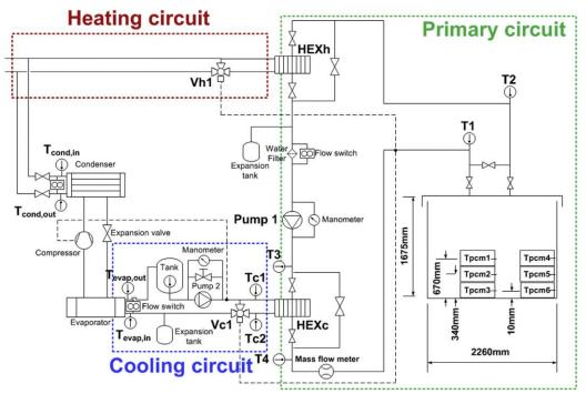
Figure 3. Schema of thermal storage system [12]
