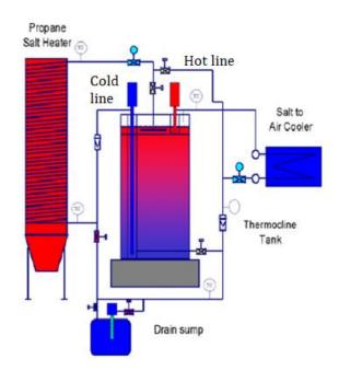
Figure 1. Thermal energy storage system with single tank. [10]
