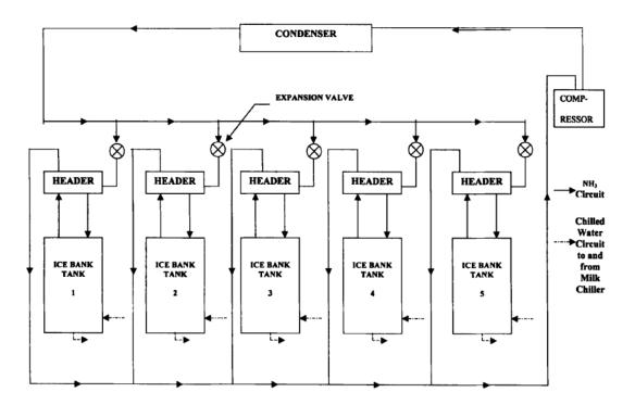
Figure 2. Scheme of thermal energy storage system in milk processing plant [6]
